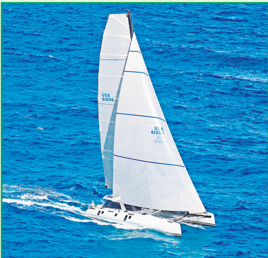
The Gunboat 60 has a beam of 28.21 feet, and drafts between 2.62 feet to 9.2 feet when the boards are lowered. Her mast is 85.40 feet tall and can displace 42,990 pounds when fully load.
